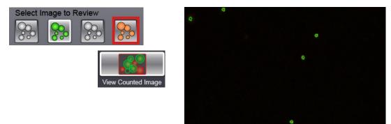
4. Tap the **View Combined Image** icon to view both the Red and Green flourescent images together. In addition, tap the **View Counted Image** icon to toggle display of the Counted graphic overlay.
