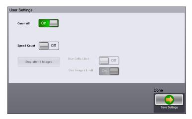
To enable speed counting, tap the **Speed Count** option and choose a parameter to limit the count: *Use Cells Limit* or *Use Images Limit*. Tap on the **Stop after...** button and use the virtual keypad to enter a number of cells or images to stop the counting process accordingly.
