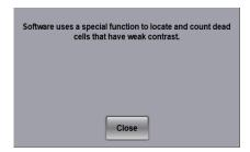
**Enhancement Value** – *Dim Dead Cell feature must be selected for this field to be enabled.* Refines the division between the background and cells with low contrast (i.e., no defined edges). *Suggested enhancement value is 0.60; values range from 0.04 (stained cells have medium contrast to background) to 0.90 (stained cells have very low contrast to background).*
